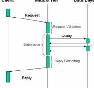
Figure 3 3-tier Sequence diagram
