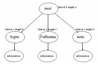
Figure 7: XML parsed document with pointer to the nodes
